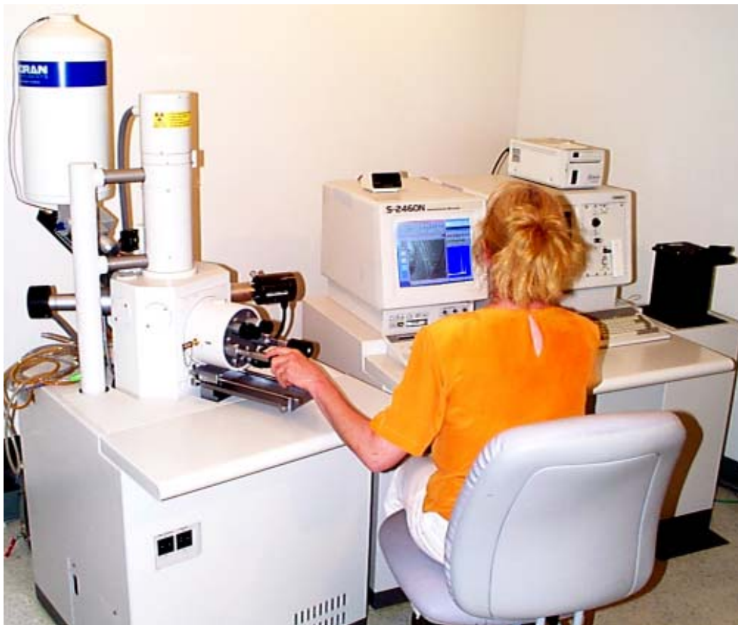
Figure 3 A scanning electron microscope (SEM) with capabilities for examining a hydrated specimen in a partial vacuum. This instrument also has X-ray analytical capabilities. A portion of the X-ray detector is shown in the top left (arrow) corner of this figure.
