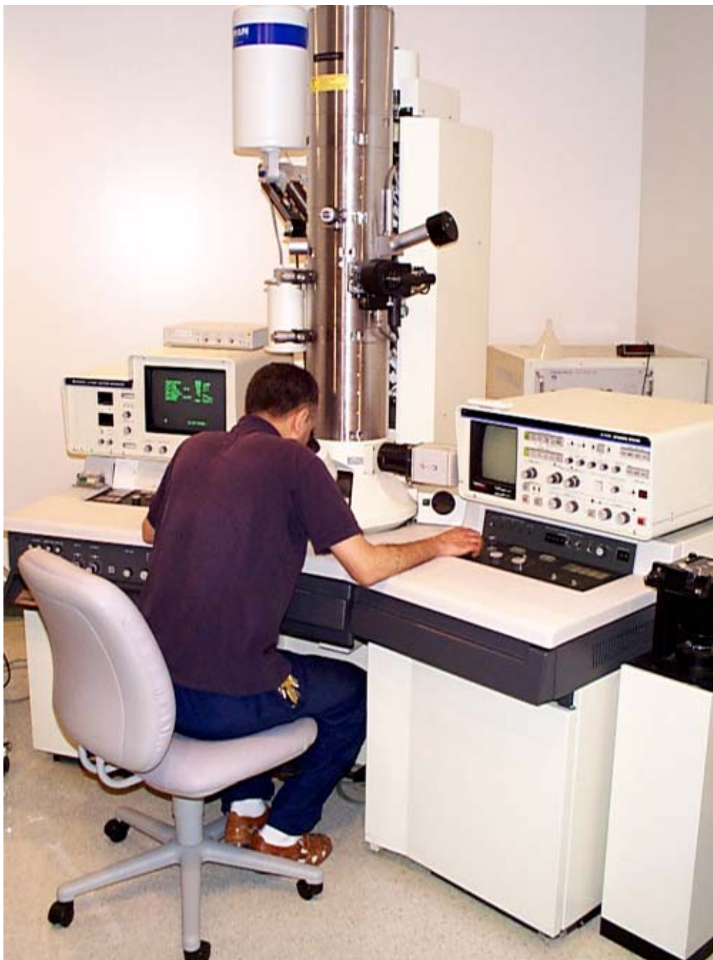
Figure 2 This modern TEM has capabilities for scanning transmission electron microscopy (STEM) and X-ray microanalysis.
